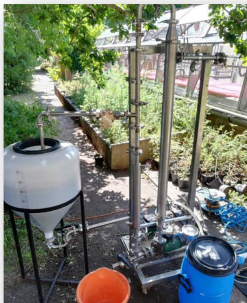
▲ Ceramic membrane set-up for ultra-filtration
