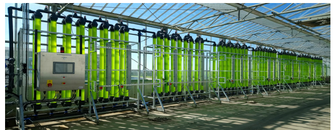
Langage photobioreactor for algal cultivation
