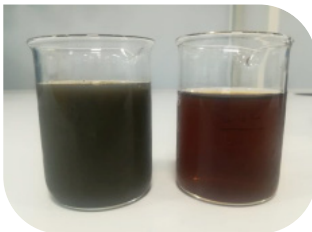
▲ Pure digestate pre ultra-filtration (left) and post micro-filtration (right)
