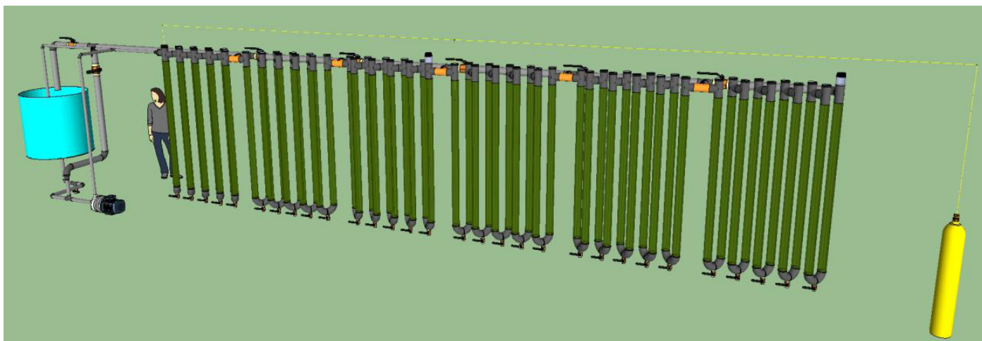
▲ Schematic representation of planned installation of algal cultivation system for Langage AD
