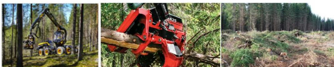
Figure 27. Left: A harvester unit is seen in operation, removing branches (grot) from a log. Right: The image depicts a fertile area dominated by spruce trees, resulting in a higher volume of GROT.
